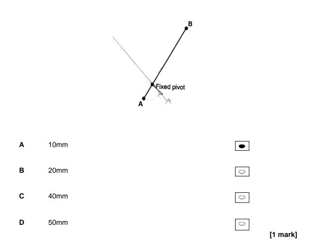
If point A moves 10mm anticlockwise about the fixed pivot, point B will move 40 mm anticlockwise. Response **C** is correct.
