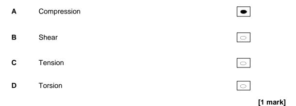
The weight of the person opposes the resistance the ground provides, hence compression is the correct answer. Response **A** is correct.
