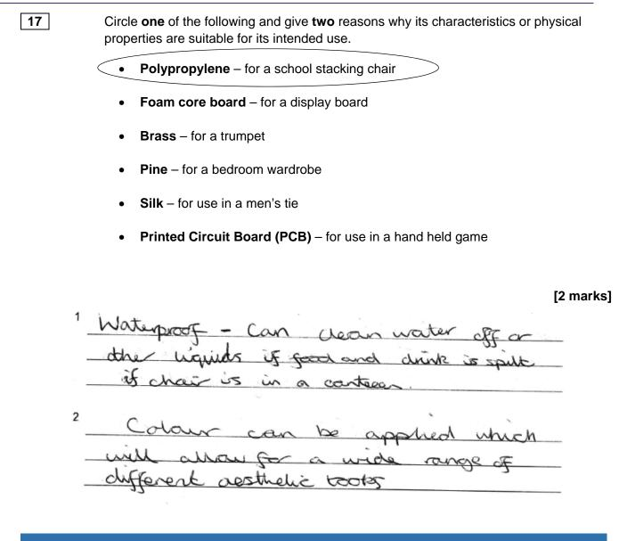
Student has selected polypropylene for a school stacking chair. There is no mark for this, but it is required to provide a focus/context for both reasons. Waterproof is fully explained (1). Colour is fully explained (1). Both these responses are very detailed and easily worth two marks.
