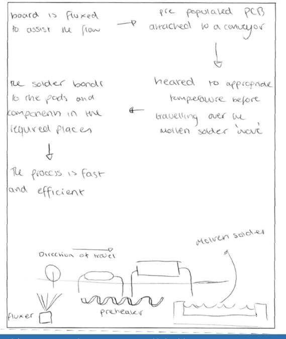
One mark for correct appropriate process – wave soldering (1). A sound response supported with a labelled diagram but some additional detail lacking in relation to mechanical movement and specific temperature (3).
