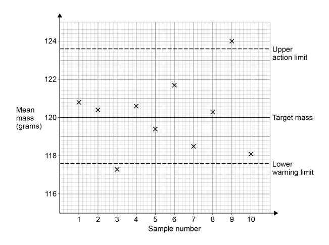
**14 (a)** The limit lines are symmetrical about the target mass.
