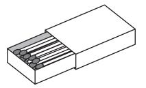
The tray and the sleeve are cut from card, folded, and glued into place using tabs. The outside faces of the tray and the sleeve are then painted to make them eye-catching.
