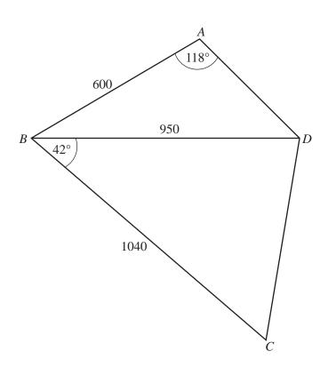
In the diagram, the quadrilateral *ABCD* represents a level park with a path *BD*.  $AB = 600 \,\text{m}$ ,  $BC = 1040 \,\text{m}$ ,  $BD = 950 \,\text{m}$ ,  $C\hat{B}D = 42^{\circ}$  and  $B\hat{A}D = 118^{\circ}$ .
