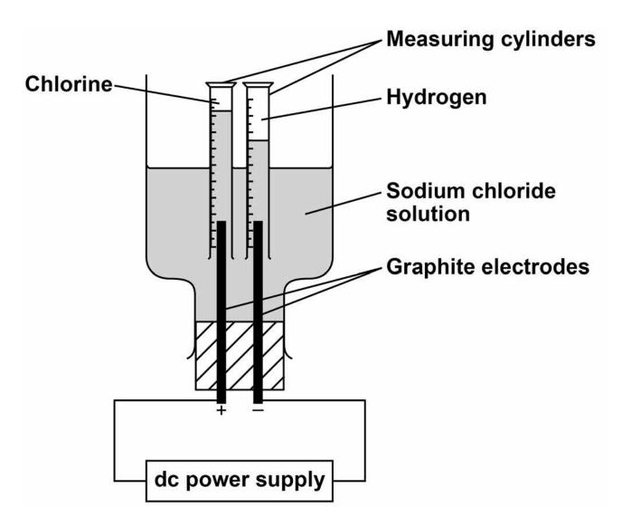
The student measured the volume of gas collected in each measuring cylinder every minute for 20 minutes.
