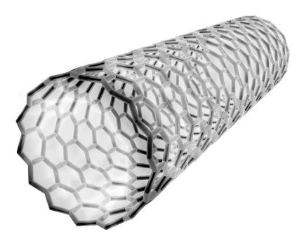
The structure and bonding in a carbon nanotube are similar to graphene.
