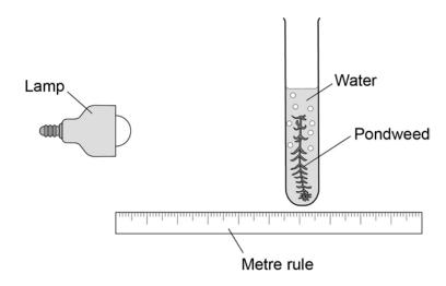
The student altered the distance of the lamp from the pondweed and counted the number of bubbles produced in 30 seconds for each distance.
