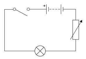
0 1. 1 To calculate power output the student measured the current in the lamp and the potential difference across the lamp.
