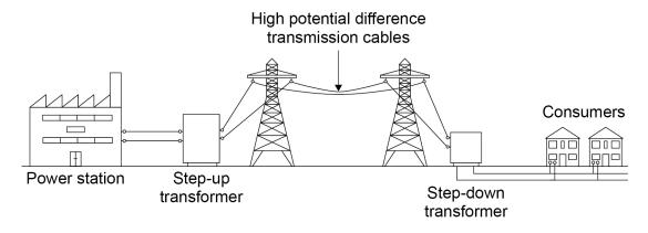
**0 2**. **1** The National Grid is a system of cables and transformers linking power stations to consumers.
