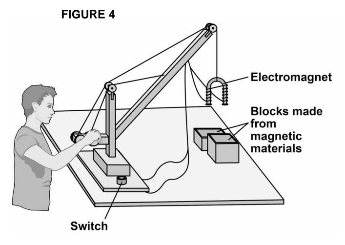
The toy crane uses an electromagnet to pick up and move the blocks.
