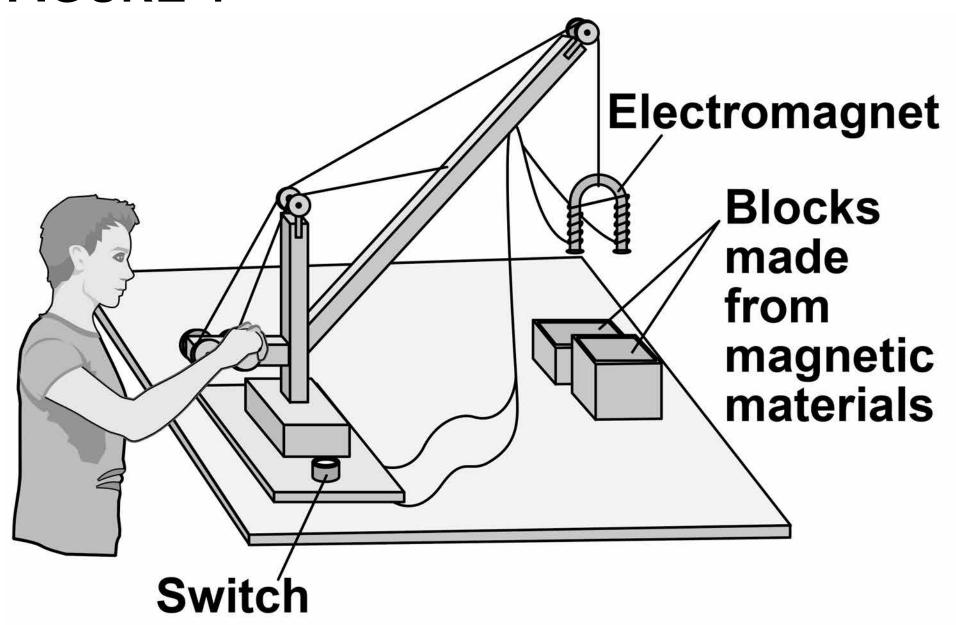
The toy crane uses an electromagnet to pick up and move the blocks.
