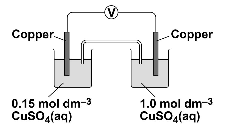
The student recorded an initial voltage of +0.16 V at 25 °C
