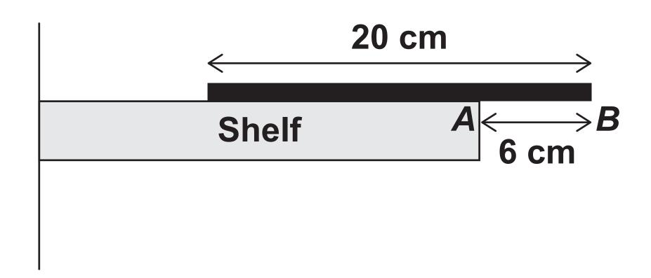
14 (a) The rod is in equilibrium when an object of mass 0.28 kilograms hangs from the midpoint of *AB*.
