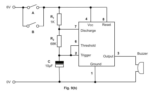
(i) State the logic function achieved by the arrangement of the two switches A and B in Fig. 9(b) and explain how this logic function is achieved. [2]
