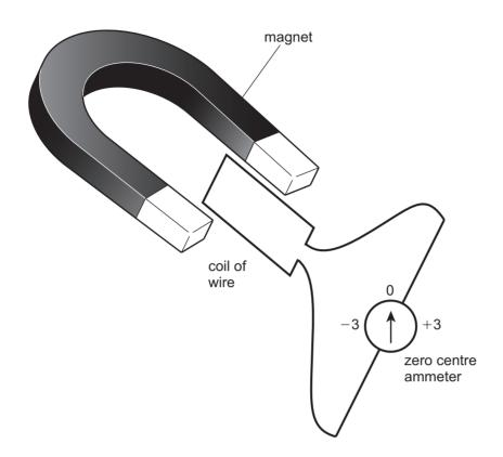
When Luke moves the coil into the gap between the poles of the magnet, the needle on the ammeter moves to -3 and returns to zero.
