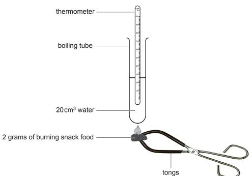
They measured the temperature of 20 cm<sup>3</sup> of water before and after **completely** burning **2 grams** of each snack food. They calculated the rise in temperature for each snack food.
