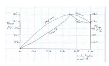
Max at 0.7/125, vapour and liquid lines labelled
