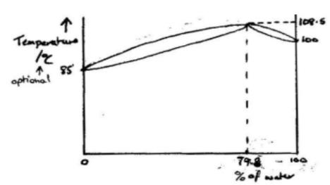
Sketch (1), axes labelled (1) correct b.p.s and azeotrope composition shown (1) Liquid and vapour curves labelled (1) Explanation of why the residue is the azeotrope (1)
