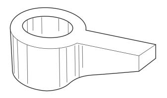
PCB drill bracket cast aluminium
