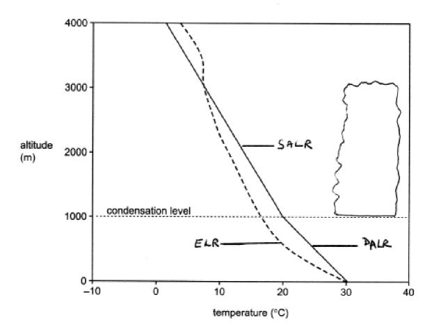
(b) On Fig. 2, draw a towering cumulus cloud showing its location and vertical extent. [2] The cloud should be flat based at condensation level and extend vertically to 3000 m
