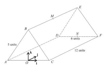
The diagram shows a triangular prism with a horizontal rectangular base ADFC, where CF = 12 units and DF = 6 units. The vertical ends ABC and DEF are isosceles triangles with AB = BC = 5 units. The mid-points of BE and DF are M and N respectively. The origin O is at the mid-point of AC.
