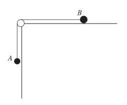
Particles A and B, of masses 0.2 kg and 0.3 kg respectively, are connected by a light inextensible string. The string passes over a smooth pulley at the edge of a rough horizontal table. Particle A hangs freely and particle *B* is in contact with the table (see diagram).
