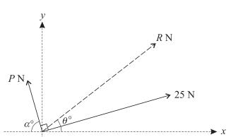
Forces of magnitudes P N and 25 N act at right angles to each other. The resultant of the two forces has magnitude R N and makes an angle of  $\theta^{\circ}$  with the x-axis (see diagram). The force of magnitude P N has components -2.8 N and 9.6 N in the x-direction and the y-direction respectively, and makes an angle of  $\alpha^{\circ}$  with the negative x-axis.
