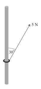
A small ring of mass  $0.6 \, \text{kg}$  is threaded on a rough rod which is fixed vertically. The ring is in equilibrium, acted on by a force of magnitude 5 N pulling upwards at  $30^{\circ}$  to the vertical (see diagram).
