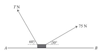
Two light strings are attached to a block of mass  $20 \,\mathrm{kg}$ . The block is in equilibrium on a horizontal surface AB with the strings taut. The strings make angles of  $60^\circ$  and  $30^\circ$  with the horizontal, on either side of the block, and the tensions in the strings are T N and 75 N respectively (see diagram).
