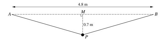
A particle P of mass 0.35 kg is attached to the mid-point of a light elastic string of natural length 4 m. The ends of the string are attached to fixed points A and B which are 4.8 m apart at the same horizontal level. P hangs in equilibrium at a point 0.7 m vertically below the mid-point M of AB (see diagram).
