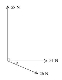
Coplanar forces of magnitudes 58 N, 31 N and 26 N act at a point in the directions shown in the diagram. Given that  $\tan \alpha = \frac{5}{12}$ , find the magnitude and direction of the resultant of the three forces.
