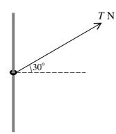
The diagram shows a ring of mass 2 kg threaded on a fixed rough vertical rod. A light string is attached to the ring and is pulled upwards at an angle of  $30^{\circ}$  to the horizontal. The tension in the string is *T* N. The coefficient of friction between the ring and the rod is 0.24. Find the two values of *T* for which the ring is in limiting equilibrium. [8]
