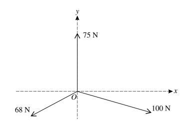
Three coplanar forces of magnitudes 68 N, 75 N and 100 N act at an origin O, as shown in the diagram. The components of the three forces in the positive x-direction are -60 N, 0 N and 96 N, respectively. Find
