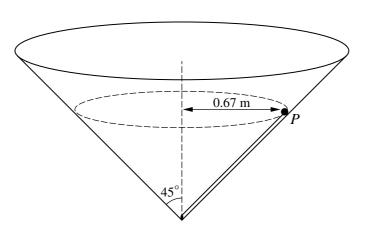
A particle P is moving inside a smooth hollow cone which has its vertex downwards and its axis vertical, and whose semi-vertical angle is 45°. A light inextensible string parallel to the surface of the cone connects P to the vertex. P moves with constant angular speed in a horizontal circle of radius 0.67 m (see diagram). The tension in the string is equal to the weight of P. Calculate the angular speed of P.
