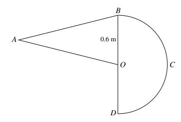
A uniform lamina OABCD consists of a semicircle BCD with centre O and radius 0.6 m and an isosceles triangle OAB, joined along OB (see diagram). The triangle has area  $0.36 \,\mathrm{m}^2$  and AB = AO.
