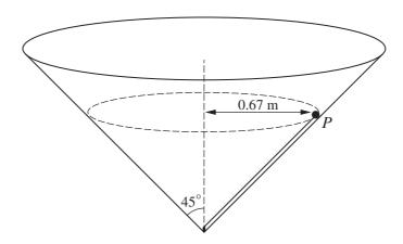
A particle P is moving inside a smooth hollow cone which has its vertex downwards and its axis vertical, and whose semi-vertical angle is 45°. A light inextensible string parallel to the surface of the cone connects P to the vertex. P moves with constant angular speed in a horizontal circle of radius  $0.67 \,\mathrm{m}$  (see diagram). The tension in the string is equal to the weight of P. Calculate the angular speed of *P*. [6]
