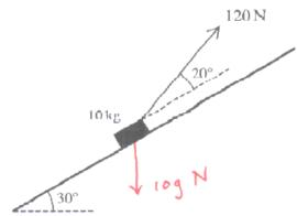
A block of mass 10 kg is at rest on a rough plane inclined at an angle of 30° to the horizontal. A force of 120 N is applied to the block at an angle of 20° above a line of greatest slope (see diagram). There is a force resisting the motion of the block and 200 J of work is done against this force when the block has moved a distance of 5 m up the plane from rest.
