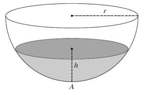
A tank containing water is in the form of a hemisphere. The axis is vertical, the lowest point is *A* and the radius is *r*, as shown in the diagram. The depth of water at time *t* is *h*. At time t = 0 the tank is full and the depth of the water is *r*. At this instant a tap at *A* is opened and water begins to flow out at a rate proportional to  $\sqrt{h}$ . The tank becomes empty at time t = 14.
