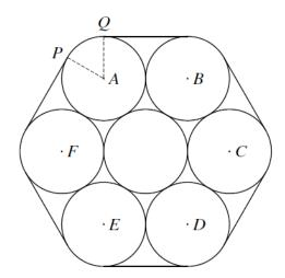
The diagram shows a cross-section of seven cylindrical pipes, each of radius 20 cm, held together by a thin rope which is wrapped tightly around the pipes. The centres of the six outer pipes are A, B, C, D, E and F. Points P and Q are situated where straight sections of the rope meet the pipe with centre A.
