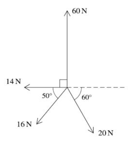
Coplanar forces of magnitudes 60 N, 20 N, 16 N and 14 N act at a point in the directions shown in the diagram.
