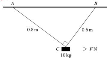
The diagram shows a block of mass  $10 \, \text{kg}$  suspended below a horizontal ceiling by two strings AC and BC, of lengths  $0.8 \, \text{m}$  and  $0.6 \, \text{m}$  respectively, attached to fixed points on the ceiling. Angle  $ACB = 90^{\circ}$ . There is a horizontal force of magnitude F N acting on the block. The block is in equilibrium.
