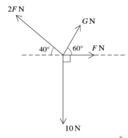
Four coplanar forces act at a point. The magnitudes of the forces are 10N, FN, GN and 2FN. The directions of the forces are as shown in the diagram.
