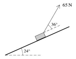
A block of mass  $12\,\mathrm{kg}$  is placed on a plane which is inclined at an angle of  $24^\circ$  to the horizontal. A light string, making an angle of  $36^\circ$  above a line of greatest slope, is attached to the block. The tension in the string is  $65\,\mathrm{N}$  (see diagram). The coefficient of friction between the block and plane is  $\mu$ . The block is in limiting equilibrium and is on the point of sliding up the plane.
