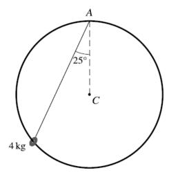
A ring of mass 4kg is threaded on a smooth circular rigid wire with centre C. The wire is fixed in a vertical plane and the ring is kept at rest by a light string connected to A, the highest point of the circle. The string makes an angle of 25° to the vertical (see diagram).
