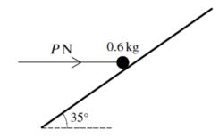
A particle of mass  $0.6 \,\mathrm{kg}$  is placed on a rough plane which is inclined at an angle of  $35^\circ$  to the horizontal. The particle is kept in equilibrium by a horizontal force of magnitude PN acting in a vertical plane containing a line of greatest slope (see diagram). The coefficient of friction between the particle and plane is 0.4.
