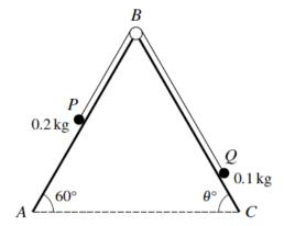
Two particles P and Q, of masses 0.2 kg and 0.1 kg respectively, are attached to the ends of a light inextensible string. The string passes over a fixed smooth pulley at B which is attached to two inclined planes. Particle P lies on a smooth plane AB which is inclined at 60° to the horizontal. Particle Q lies on a plane BC which is inclined at an angle of  $\theta$ ° to the horizontal. The string is taut and the particles can move on lines of greatest slope of the two planes (see diagram).
