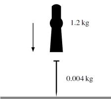
A machine for driving a nail into a block of wood causes a hammerhead to drop vertically onto the top of a nail. The mass of the hammerhead is 1.2 kg and the mass of the nail is 0.004 kg (see diagram). The hammerhead hits the nail with speed  $v \text{ m s}^{-1}$  and remains in contact with the nail after the impact. The combined hammerhead and nail move immediately after the impact with speed  $40 \text{ m s}^{-1}$ .
