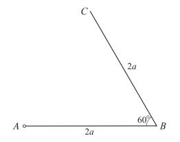
Two uniform rods AB and BC, each of length 2a and mass m, are rigidly joined at B so that angle  $ABC = 60^{\circ}$  (see diagram). The system is free to rotate in a vertical plane about a horizontal axis though A. Show that the moment of inertia of the system about this axis is  $\frac{14}{3}ma^2$ . [3]
