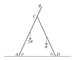
The diagram shows a pair of stepladders modelled by two uniform rods, AB of length 5a and weight 2W and CD of length 4a and weight W, smoothly hinged at C. The stepladders rest on a rough horizontal floor with A fixed so that it cannot slide. The angles CAD and CDA are both equal to  $\alpha$ . By taking moments about A for the system, find the normal contact force at D. [3]
