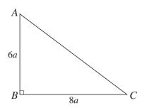
A uniform wire, of length 24a and mass m, is bent into the form of a triangle ABC with angle  $ABC = 90^{\circ}$ , AB = 6a and BC = 8a (see diagram). Find the moment of inertia of the wire about an axis through A perpendicular to the plane of the wire.
