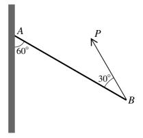
A uniform rod AB of weight W rests in equilibrium with A in contact with a rough vertical wall. The rod is in a vertical plane perpendicular to the wall, and is supported by a force of magnitude P acting at B in this vertical plane. The rod makes an angle of  $60^{\circ}$  with the wall, and the force makes an angle of  $30^{\circ}$  with the rod (see diagram). Find the value of *P*. [3]
