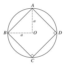
A rigid body is made from uniform wire of negligible thickness and is in the form of a square ABCD of mass M enclosed within a circular ring of radius a and mass 2M. The centres of the square and the circle coincide at O and the corners of the square are joined to the circle (see diagram). Show that the moment of inertia of the body about an axis through O, perpendicular to the plane of the body, is  $\frac{8}{3}Ma^2$ .
