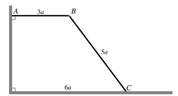
Two uniform rods AB and BC are smoothly jointed at B and rest in equilibrium with C on a rough horizontal floor and with A against a rough vertical wall. The rod AB is horizontal and the rods are in a vertical plane perpendicular to the wall. The rod AB has mass 3m and length 3a, the rod BC has mass 5m and length 5a, and C is at a distance 6a from the wall (see diagram). Show that the normal reaction exerted by the floor on the rod BC at C has magnitude  $\frac{13}{2}mg$ .
