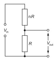
Which expression gives the ratio of  $\frac{V_{\text{out}}}{V_{\text{in}}}$ ?
