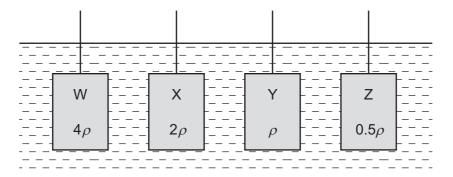
Water has density  $\rho$ . Cuboid W is made of material of density  $4\rho$ . Cuboid X is made of material of density  $2\rho$ . Cuboid Y is made of material of density  $\rho$ . Cuboid Z is made of material of density  $0.5\rho$ .
