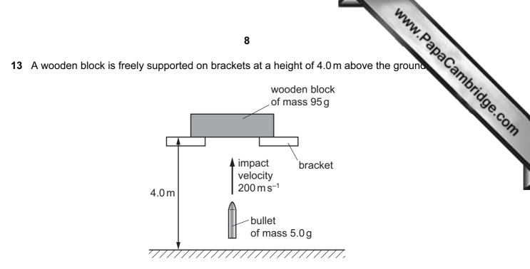
A bullet of mass 5.0 g is shot vertically upwards into the wooden block of mass 95 g. It embeds itself in the block. The impact causes the block to rise above its supporting brackets.
