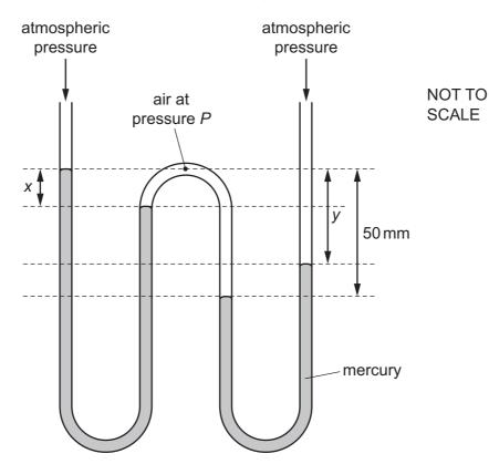
Atmospheric pressure is equal to the pressure that would be exerted by a column of mercury of height 760 mm. The pressure *P* is expressed in this way.
