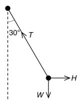
The tension in the string of the pendulum is T. The weight of the pendulum bob is W.
