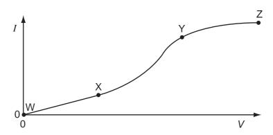
In which ways does the resistance of the component vary within each of the three sections?
