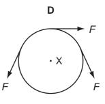
15 Three coplanar forces, each of magnitude 10 N, act through the same point of a body in the directions shown.
