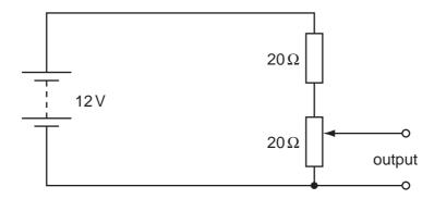
The fixed resistor and the potentiometer each have resistance 20  $\Omega$ . The circuit is designed to provide a variable output voltage.
