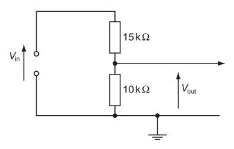
$V_{\rm out}$  is equal to 4.8 V.
