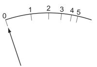
The ammeter is accidentally readjusted so that when the current is zero, the pointer is at X.
