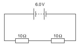
What charge flows through each of the  $10\Omega$  resistors in 1 minute?
