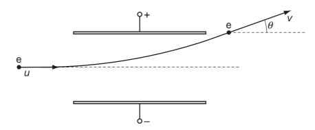
While in the electric field, its direction changes by  $\theta$  and it emerges with a velocity  $\nu$ .
