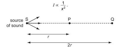
Air molecules at P, a distance r from S, oscillate with amplitude 8.0  $\mu$ m.
