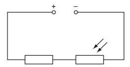
When the LDR is in the dark, the fixed resistor and the LDR have the same value of resistance.
