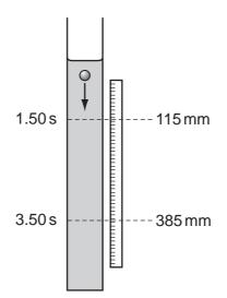
There are two marks on the tube. The top mark is positioned at  $115 \pm 1$  mm on the adjacent rule and the lower mark at 385  $\pm$  1 mm. The ball passes the top mark at 1.50  $\pm$  0.02 s and passes the lower mark at  $3.50 \pm 0.02 \, s$ .
