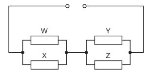
How will the powers to the resistors change when resistor W is removed?
